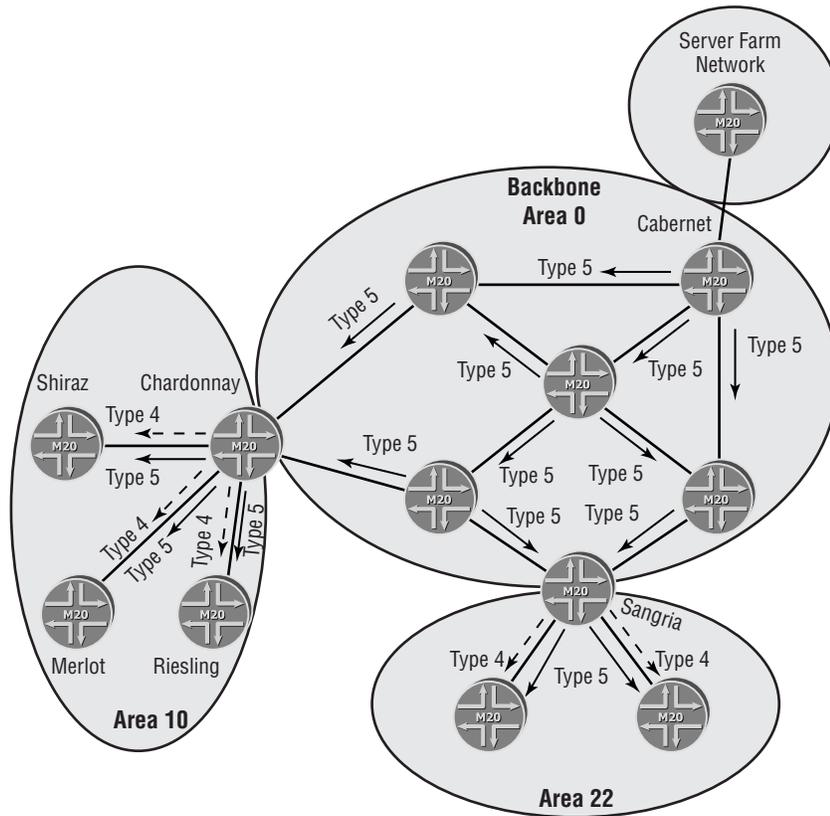
While the Type 5 LSA provides the network information necessary to reach the external networks, the OSPF routers may not automatically begin using that data. The address of the ASBR, Cabernet in our case, must be known in the link-state database via a router LSA. Chardonnay, Sangria, and the other backbone routers meet this criterion, because they share an area 0 database with Cabernet. It is the routers in area 10 and 22 that are currently not able to utilize the AS external LSA.
