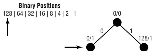
At the first position, the first octet of the IP address has a value of 00000000 or 10000000—a 0 or 128, respectively. This is represented in Figure 4.6 by the values 0 /1 and 128 /1. The second step of the tree is shown in Figure 4.7.
