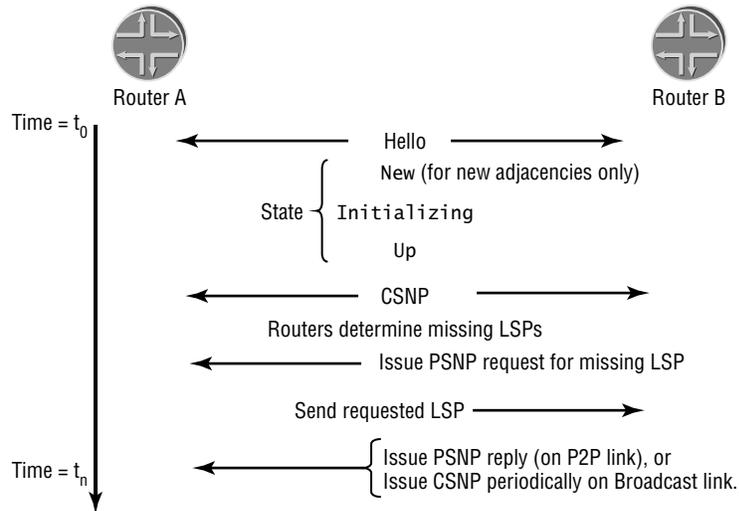
Router A and Router B are forming an adjacency and exchanging the information in their databases. The specific steps of this process are:
