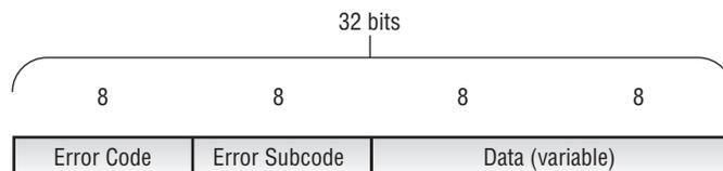
In addition to the common BGP header, the Notification message contains the following:
