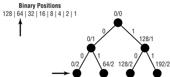
This second level of the tree has four possible binary values for the first octet: 00000000, 01000000, 10000000, and 11000000. These decimal values of 0, 64, 128, and 192 are represented by the IP addresses of 0 /2, 64 /2, 128 /2, and 192 /2 on the radix tree. This step-by-step
