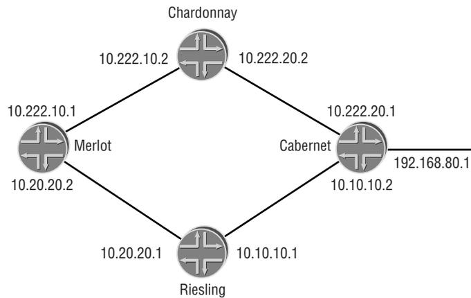
The currently assigned next hop for 192.168.80.1 /32 is Riesling’s interface of 10.20.20.1. Recall from the “JUNOS software Routing Table” section earlier in this chapter that a caret marker (>) designates the next hop installed in the forwarding table. The captures from Merlot clearly show this correlation. To install both 10.20.20.1 and 10.222.10.2 as next hops, we configure the following policy:
