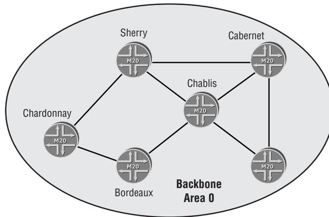
The Chablis router in area 0 is a backbone router with all interfaces within the area. This allows you to configure OSPF using two commands:
