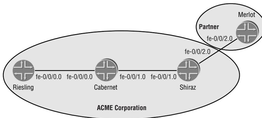
Merlot is able to communicate using the RIPv1 specification only, so Shiraz has added both the *send* and *receive* options within its *neighbor* statement for Merlot:
