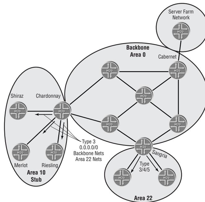
A closer examination of Figure 6.17 also reveals that Chardonnay is no longer generating ASBR summary LSAs as well. Recall from the “Non-OSPF Routes” section earlier in this chapter that the Type 4 LSAs allow OSPF routers simply to use the AS external LSAs in their databases. In a stub environment, the Type 5 LSAs are not present in the area routers, so the need for the ASBR summary LSAs is moot. The ABR, therefore, stops generating those LSAs as well.
