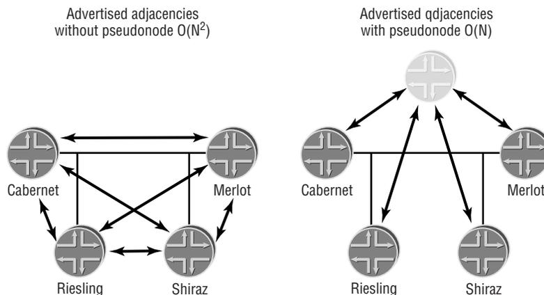
Within IS-IS, the elected pseudonode is called the DIS. The election process is very deterministic since the router with the best (highest) criteria is always the DIS. The first criterion checked is the advertised *DIS priority* of the router. The priority range is between 0 and 127, with a JUNOS software default of 64. When two or more nodes share priority values, the second criterion checked is the MAC address of the advertising router.
