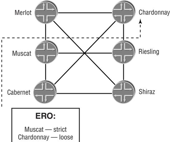
In this case, only a single strict hop is configured. Cabernet, the ingress router, finds that Muscat is directly connected and forwards the Path message to the next hop. Muscat examines the ERO and finds that the next hop is loosely defined. It then uses its IGP routing table to forward the Path message. In this example, it arrives at Riesling. Riesling performs a routing lookup to find the loose hop and forwards the Path message to Chardonnay.
