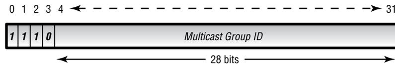
As is the case with the address space used for unicast transmissions, certain portions of the multicast group addresses are reserved for special purposes. One such group is all addresses within the 224.0.0.0 /24 subnet. These groups are restricted to a local physical media, which means that a router does not forward the datagram to other portions of the network. We enforce this restriction by setting the Time-to-Live (TTL) field to the value 1.
