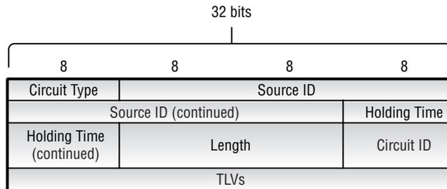
The IS-IS point-to-point Hello PDU consists of the following fields:
