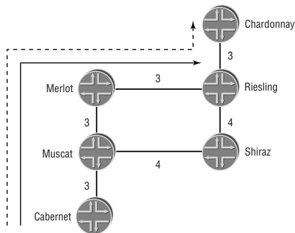
**FIGURE 11.2** IGP-based traffic engineering
