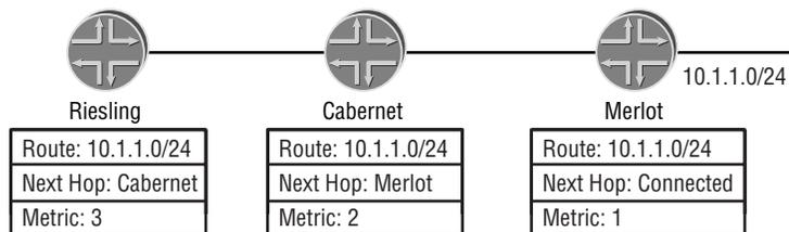
Merlot advertises the 10.1.1.0 /24 subnet to Cabernet with a metric of 1, which is in turn advertised to Riesling with a metric of 2. At this point, all three of the routers have converged on a common view of the network.
