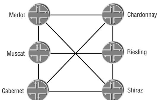
At first glance, this looks like a regular IGP-routed core with faster interfaces. However, the addition of MPLS as an operating protocol greatly alters the operation of the network. Each router now has the ability to create a label switched path (LSP) to any other router in the network. This path can traverse any number of physical links in the network.
