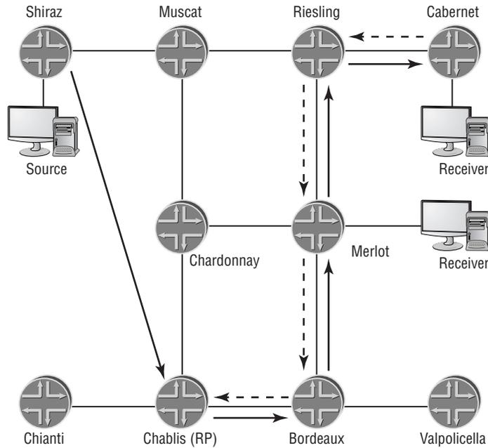
As Merlot and Cabernet begin to receive the multicast traffic, they examine the source of the multicast traffic and find that it is the host connected to Shiraz. Each router then determines whether the current forwarding path is its best path to the source, and neither router finds this to be the case. Both Merlot and Cabernet then send a request to the multicast source itself, asking for the group data stream to be sent to them directly.
