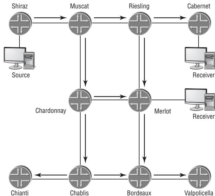
A quick look at Figure 9.9 shows that every router in the network doesn't need to receive the data stream. Only Merlot, Cabernet, and the routers along the path back to the source should be forwarding the traffic. Any router in a dense-mode network may prune itself from the forwarding path by sending a message to its upstream peer. This process occurs for all routers that do not need to receive the traffic.
