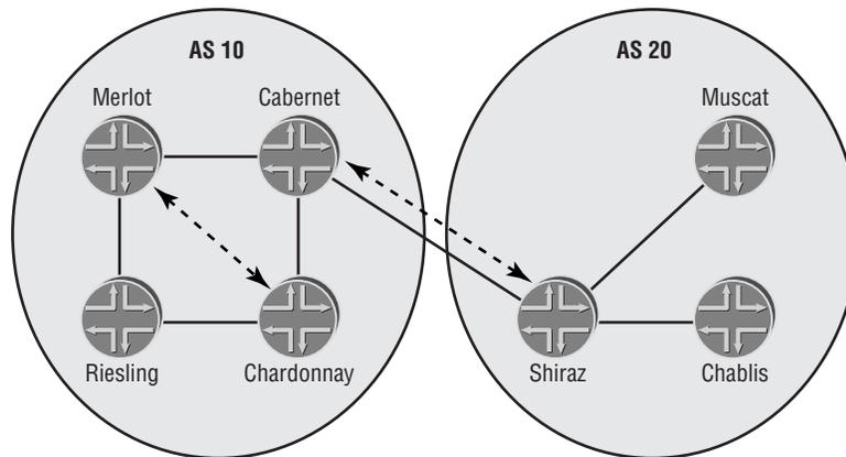
The Cabernet and Shiraz routers are joined by a direct physical connection. This connectivity implies that IP reachability is easily achieved between the two peers and that TCP can establish its session. On the other hand, the Merlot and Chardonnay routers are connected only via an intermediate router. In this situation, IP reachability between the peers must be supplied by some other means. Often this is handled by the IGP within the AS, but a static route is also a feasible solution.
