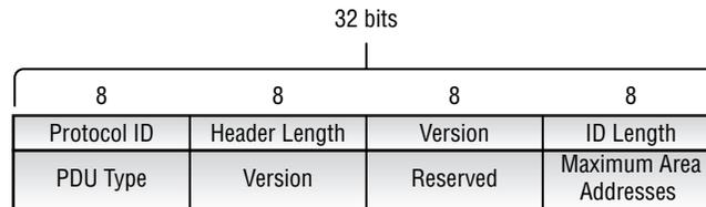
Each PDU shares a common header, illustrated in Figure 7.7. The header consists of the following fields:
