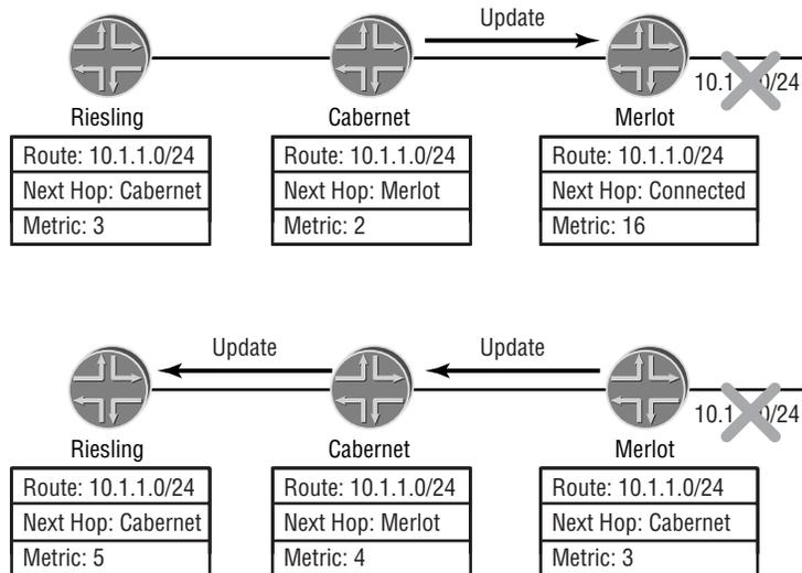
This cycle will continue until the defined infinity metric (16) is reached. At that point, all routers will agree that the 10.1.1.0/24 subnet is unreachable and will remove it from their routing tables. Until that time, however, user data packets will still be forwarded based on this false information.
