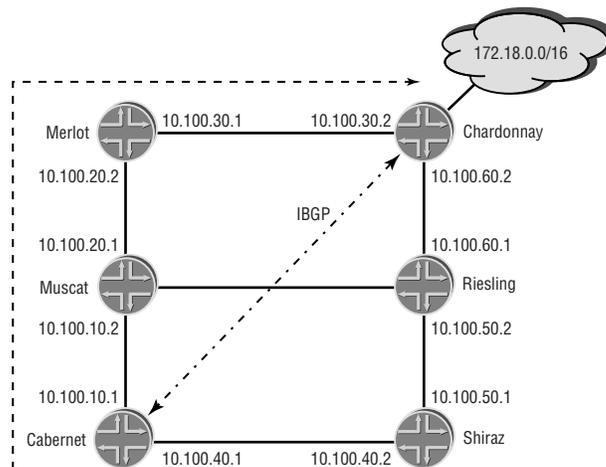
The Cabernet router is peering with Chardonnay using IBGP routing. The 172.18.0.0/16 route is advertised to Cabernet over this connection. The current BGP next-hop value is 192.168.4.4, the loopback address of Chardonnay. We can verify this information by using the `show route receive-protocol` command on Cabernet:
